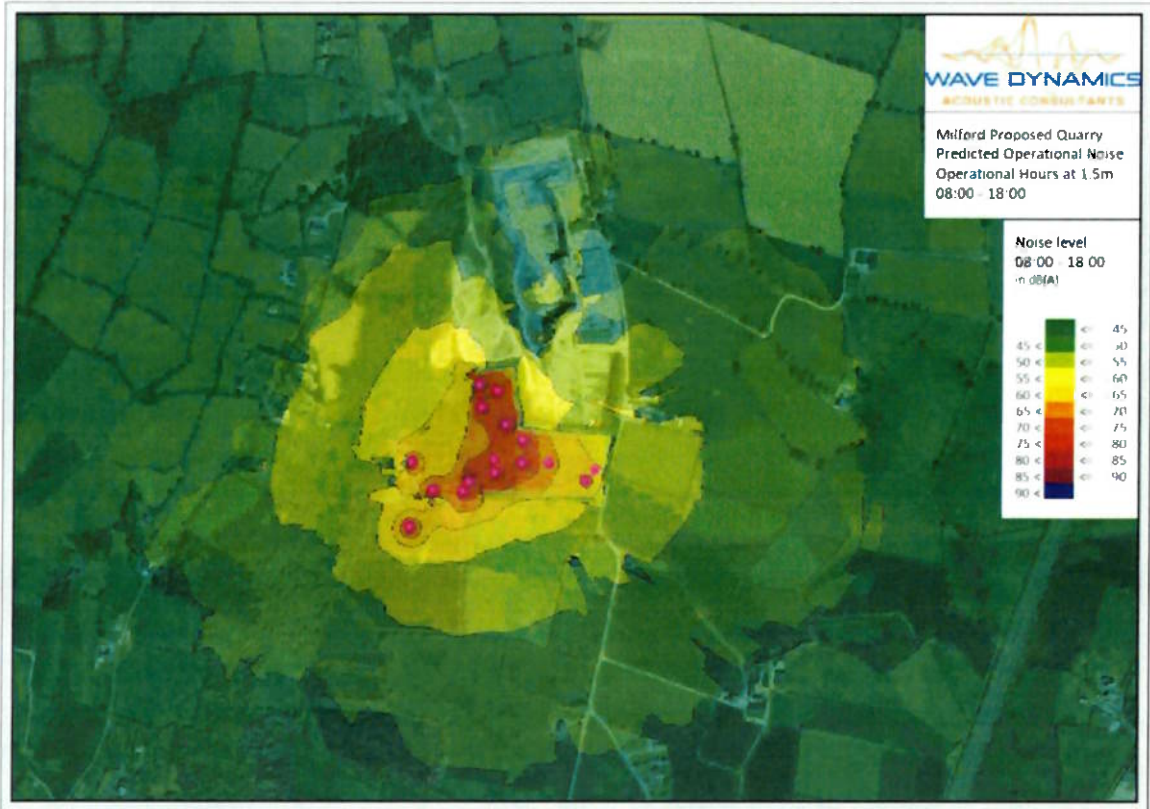
Figure 3: Grid noise map of the proposed quarry at 1.5m during operational hours.
